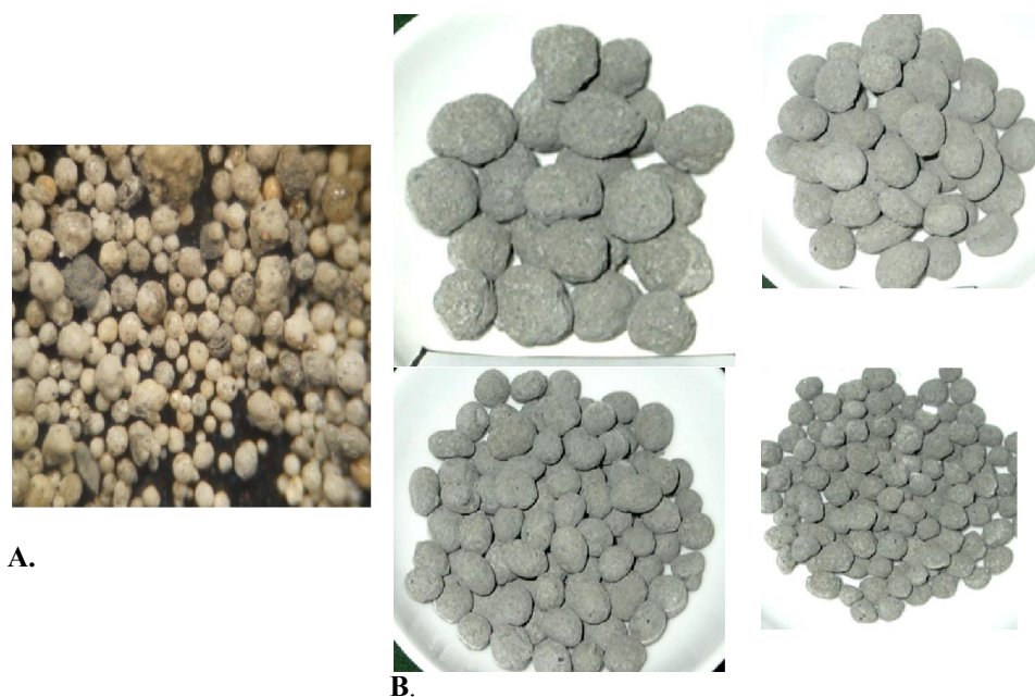
Figure 1. A. Microphotograph of light fraction of the fly ash (hollow microsphere density < 1.00 \text{ g/cm}^3 ); B. Pelletized fly ash in different size fractions
