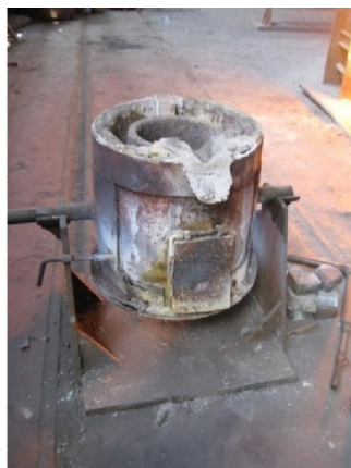
Figure 5. Soldering alloy refinement pot
