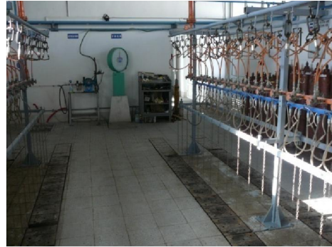
Picture 4. Scales for measuring full bottles of acetylene
