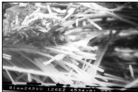
Figure 5. Fracture of fibers for GE-2 specimen (126 X)
