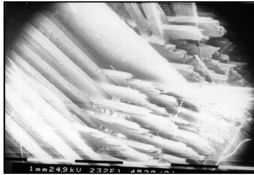
Figure 4. Fracture of fibers for GE-1 specimen (23,2 X)
