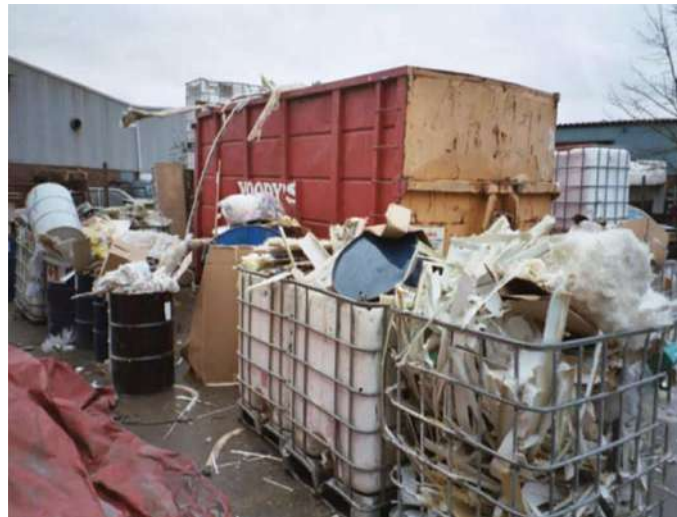
Figure 2. Disposal of waste FRP
