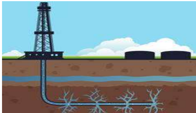
Figure 2. Scheme hydraulic fracturing method for shale gas Source:Energy.gov ( Ziare.com)
