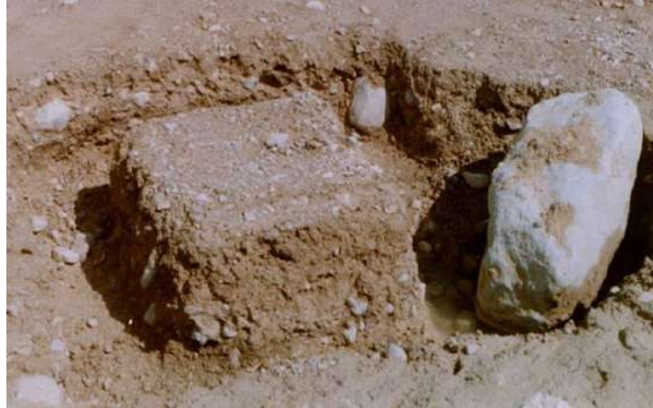
Figure 2. Sample for direct shear test [5].
